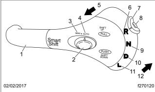
To upshift manually, pull the lever back (towards the driver). To downshift manually, push the lever forward (away from the driver).
