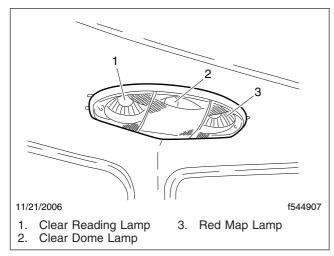
Fig. 5.9, Overhead Console Lights
