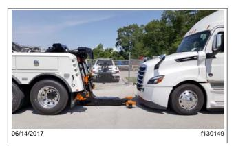
Fig. 24.8, Positioning the Stinger Assembly
