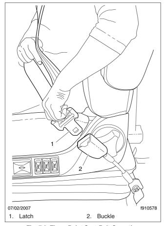
Fig. 7.9, Three-Point Seat Belt Operation
