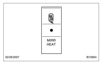
Fig. 9.2, Mirror Heat Switch
