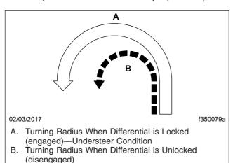
Fig. 16.1, Turning Radius
