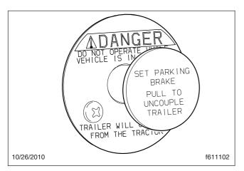
Fig. 18.10, Air-Actuated Kingpin Release Valve
