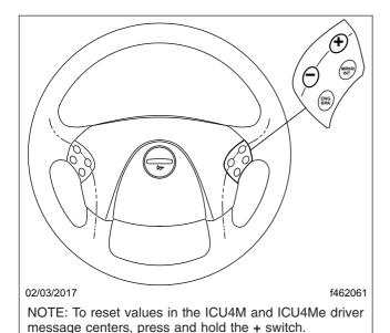
Fig. 4.11, Steering Wheel-Mounted Switches
