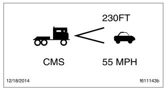
Fig. 6.20, CMS Lead Vehicle Detected (green)
