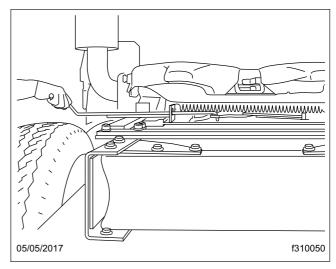
Fig. 18.12, Releasing the Sliding Fifth Wheel, (Fontaine)
