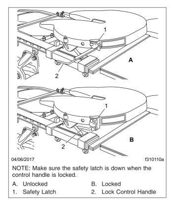
Fig. 18.2, Fontaine Locking Mechanism
