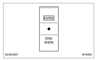
Fig. 11.2, Shutdown Override Switch
