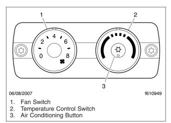
Fig. 8.5, Sleeper Climate Control Panel
