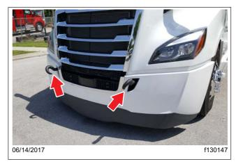
Fig. 24.7, Tow Hooks Installed, Facing Down
