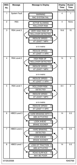
Fig. 6.39, Roll Stability and Hard-Braking Warnings
