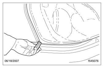
Fig. 23.4, Headlight Adjusting
