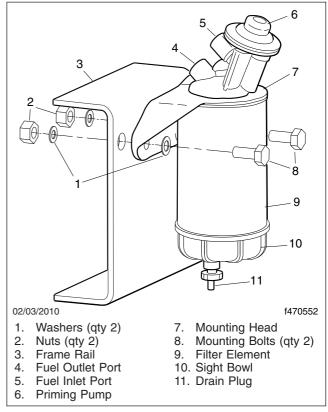
Fig. 21.16, Alliance Fuel/Water Separator Assembly and Installation
