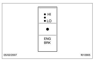
Fig. 13.6, Engine Brake Level Switch
