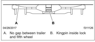
Fig. 18.6, Coupling Inspection
