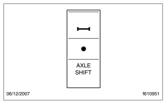
Fig. 16.2, Axle Shift Switch
