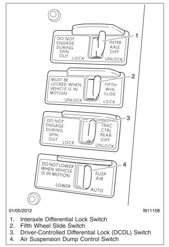
Fig. 5.15, Axle and Suspension Switches
