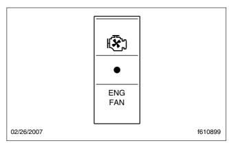
Fig. 5.17, Engine Fan Switch
