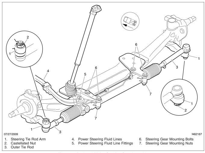
Fig. 21.19, Rack and Pinion Steering Gear Assembly
