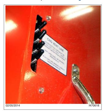
Fig. 21.9, CNG Vent Line Caps
