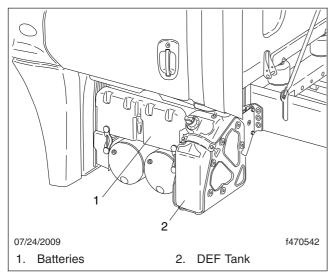
Fig. 12.7, DEF Tank Located Behind the Battery Box
