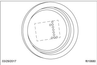
NOTE: The gear indicator displays the current gear. In this example it displays first gear.
