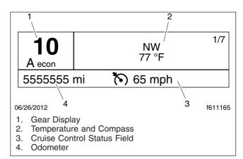
Fig. 4.24, Driver Message Center with Gear Display, ICU4Me
