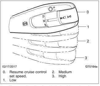
Fig. 5.27, Deceleration Mode Positions, Detroit **Multifunction Control**
