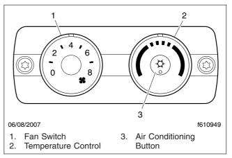
Fig. 5.38, Sleeper Climate Control Panel
