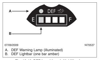
Fig. 12.10, DEF Level Low Initial Warning
