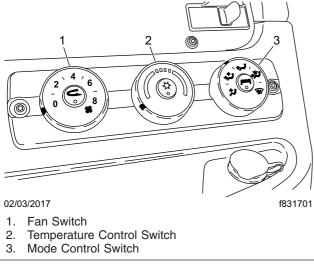
Fig. 8.1, Cab Climate Control Panel
