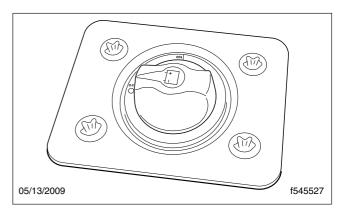
Fig. 3.7, Cab Load Disconnect Switch, EPA10 and
