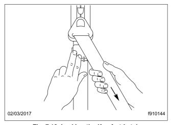
Fig. 7.12, Locking the Komfort Latch
