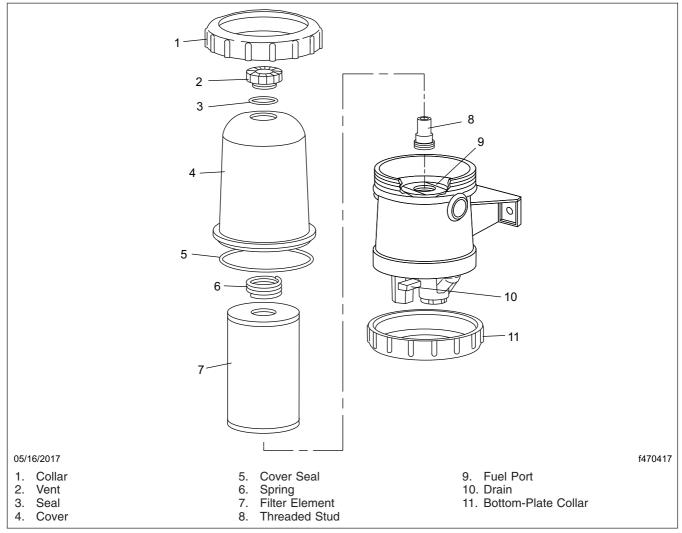
Fig. 24.2, Davco Model 382 Fuel/Water Separator
