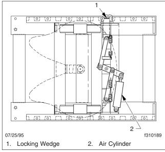
Fig. 18.15, Air-Operated Sliding Fifth Wheel (Fontaine shown)
