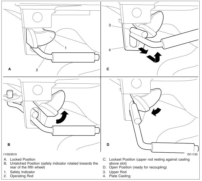
Fig. 18.9, Holland Kingpin Locking Mechanism
