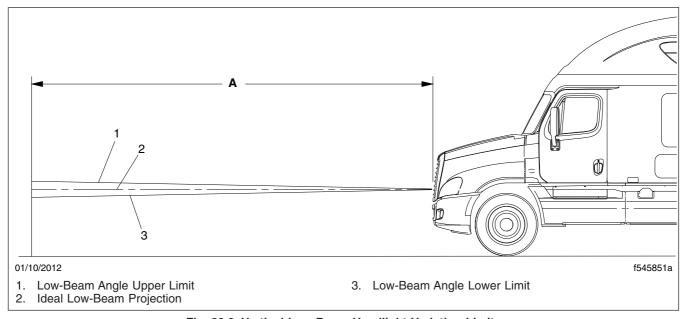
Fig. 23.3, Vertical Low-Beam Headlight Variation Limits
