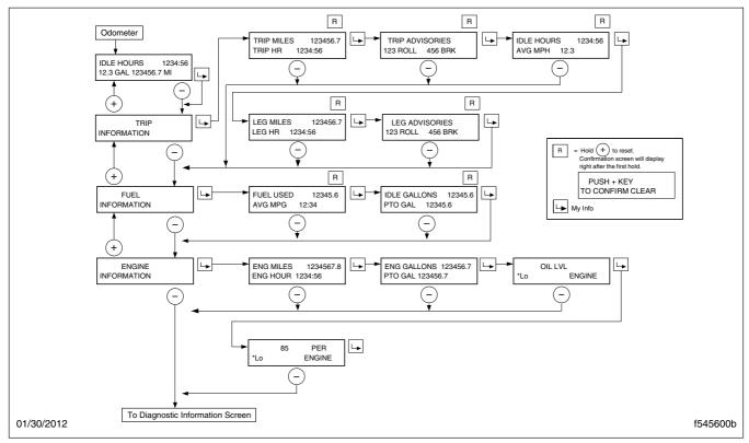
Fig. 4.18, ICU4M Idle Hours, Trip Information, Fuel Information, and Engine Information Screens
