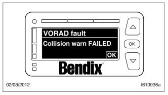
Fig. 6.15, VORAD Fault Display
