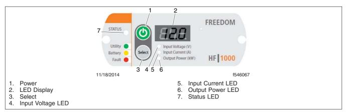
Fig. 3.10, Inverter/Charger Display Panel (1000W shown)
