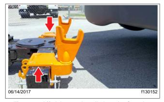
Fig. 24.12, Lift Adaptors Installed on the Crossbar
