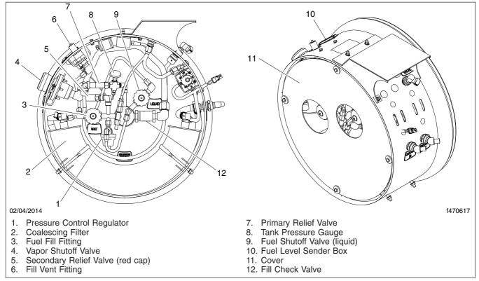
Fig. 21.10, LNG Tank Plumbing Components
