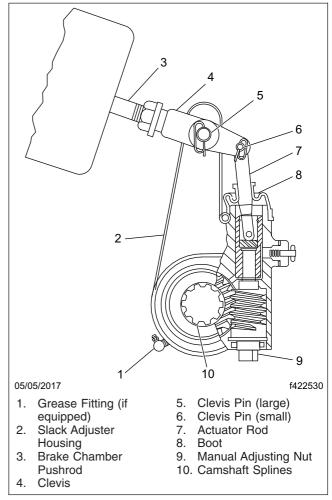
Fig. 21.3, Meritor Automatic Slack Adjuster
