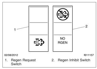
Fig. 12.1, Regen Request and Inhibit Switches
