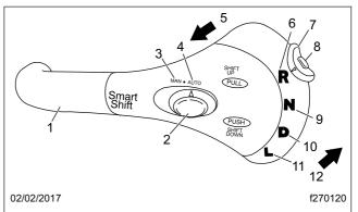
To upshift manually, pull the lever up (towards you). To downshift manually, push the lever down (away from you).
