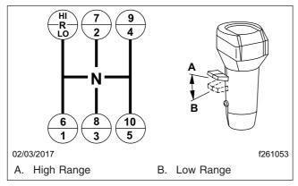
Fig. 14.3, Eaton Fuller 10-Speed Transmission Shift Patterns
