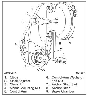
Fig. 21.2, Haldex Automatic Slack Adjuster
