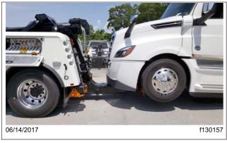
Fig. 24.17, Final Towing Position
