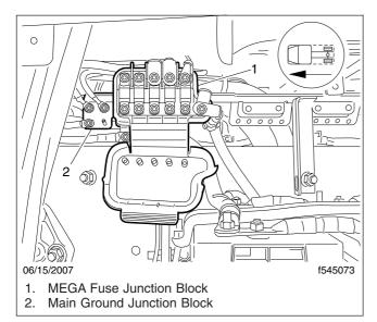
Fig. 3.2, EPA07 MEGA Fuse Junction Block
