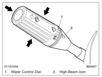
Fig. 5.8, Multifunction Turn Signal Lever
