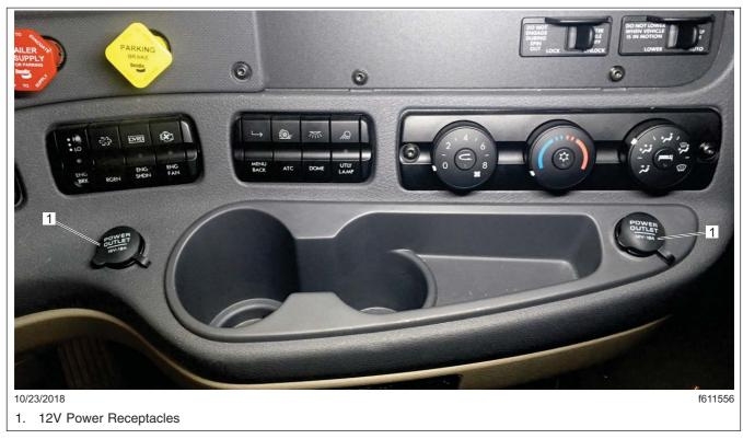
Fig. 3.8, 12V Power Receptacle, Main Dashboard
