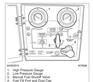
Fig. 25.3, CNG Under Cabinet Fuel Panel (under cabinet shown)
