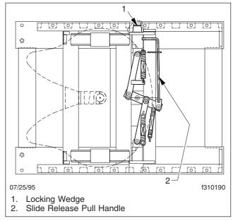
Fig. 18.11, Manual Release Sliding Fifth Wheel (Fontaine shown)
