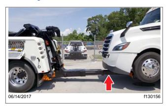
Fig. 24.16, Retracting the Recovery Boom
