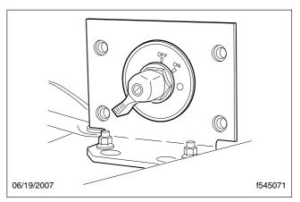
Fig. 3.6, Cab Load Disconnect Switch, EPA07
