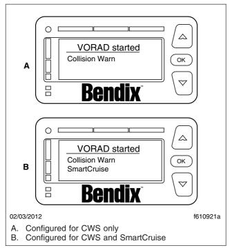
Fig. 6.2, System Configuration Screens
