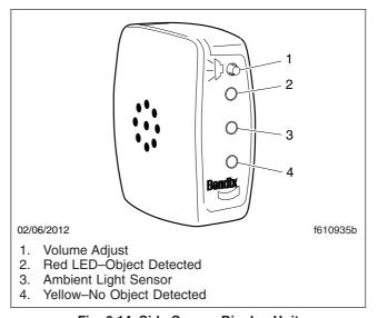
Fig. 6.14, Side Sensor Display Unit
