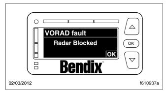
Fig. 6.16, Antenna Blocked Display
