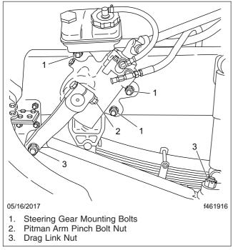
Fig. 21.20, Integral Steering Gear Fasteners
