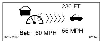
Fig. 6.23, ACC Lead Vehicle Detected (green)
