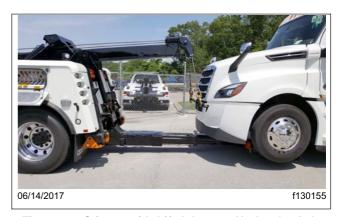
Fig. 24.15, Stinger with Lift Adaptors Under the Axle (tow truck shown)
