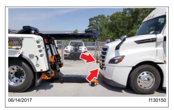
Fig. 24.10, Tow Cables Connected to the Tow Hooks
