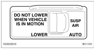
Fig. 18.1, Air-Suspension Dump Valve
