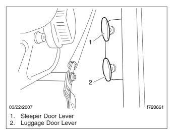
Fig. 2.6, Sleeper Door Levers
