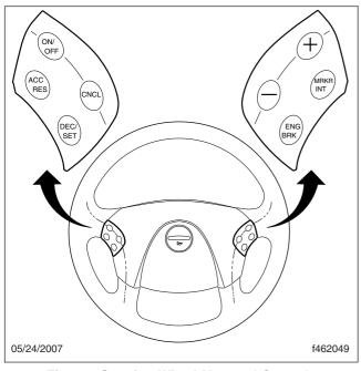
Fig. 5.7, Steering Wheel-Mounted Controls
