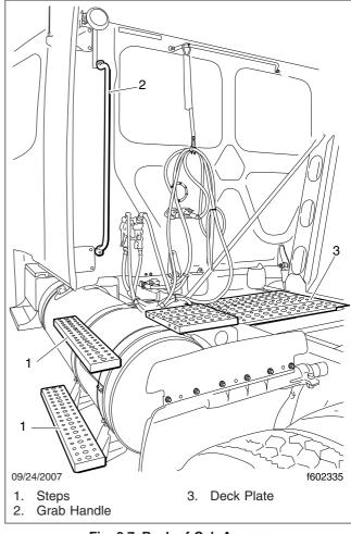
Fig. 2.7, Back-of-Cab Access
