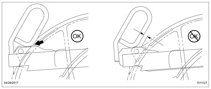
Fig. 18.8, Jost Release Handle Locked
