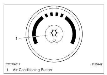
Fig. 8.3, Temperature Control Switch
