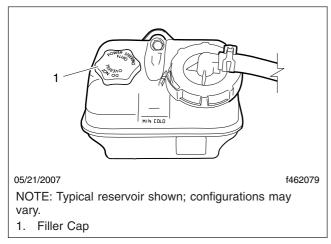
Fig. 21.5, Power Steering Fluid Reservoir
