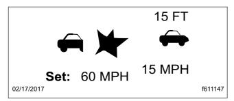
Fig. 6.24, ACC Collision Warning (red)
