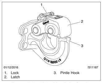
Fig. 19.1, Holland PH-10RP41 Trailer Coupling
