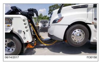
Fig. 24.18, Safety Chains Connected on the Towed Vehicle
