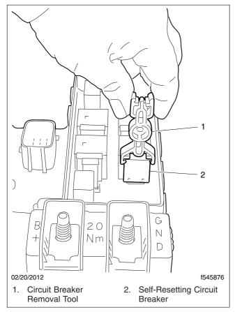
Fig. 3.5, Self-Resetting Circuit Breaker Removal
