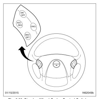
Fig. 6.28, Steering Wheel Cruise Control Switches
