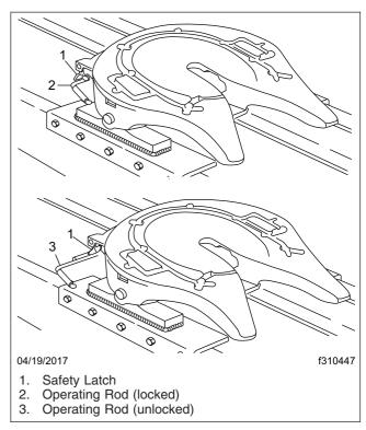
Fig. 18.3, Holland Simplex SE Locking Mechanism
