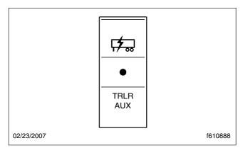
Fig. 5.35, Trailer Auxiliary Switch
