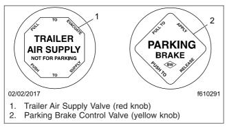
Fig. 5.28, Brake Valve Control Knobs
