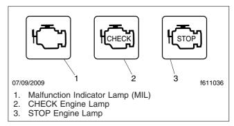
Fig. 11.1, Engine Warning Lamps
