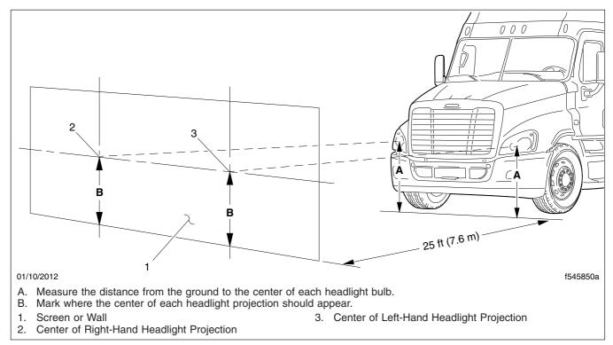
Fig. 23.2, Headlight Aiming Screen/Wall
