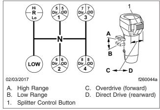
Fig. 14.1, Eaton Fuller 13-Speed Transmission Shift Pattern
