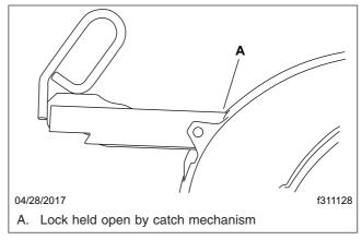
Fig. 18.7, Jost Release Handle Unlocked
