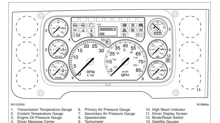
Fig. 4.1, ICU3 Instrument Cluster (EPA10 shown)
