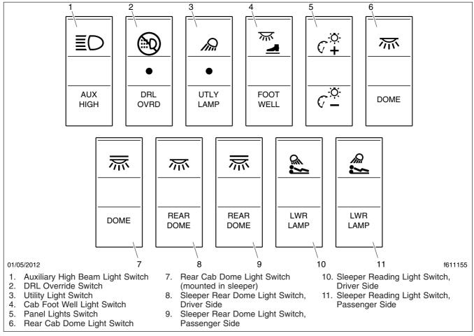
Fig. 5.4, Dash-Mounted and Sleeper-Control Light Switches
