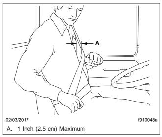
Fig. 7.11, Adjusting Shoulder Harness Clearance, Komfort Latch
