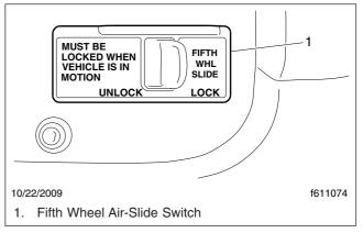
Fig. 18.14, Air-Slide Switch
