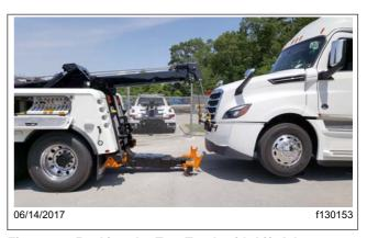
Fig. 24.13, Backing the Tow Truck with Lift Adaptors on the Crossbar
