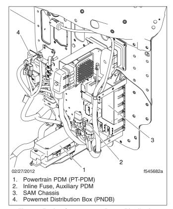
Fig. 3.3, Engine Compartment Power Distribution Components
