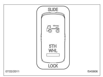
Fig. 5.34, Fifth Wheel Slide Control Switch
