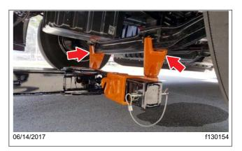
Fig. 24.14, Positioning the Stinger with Lift Adaptors
