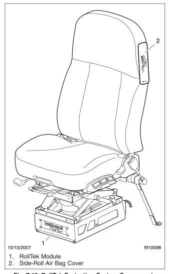
Fig. 7.13, RollTek Protection System Components
