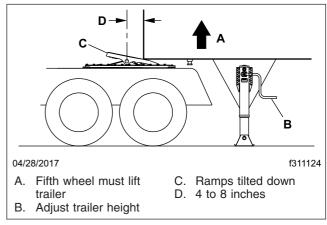
Fig. 18.4, Trailer Connection Point, Standard Fifth Wheel
