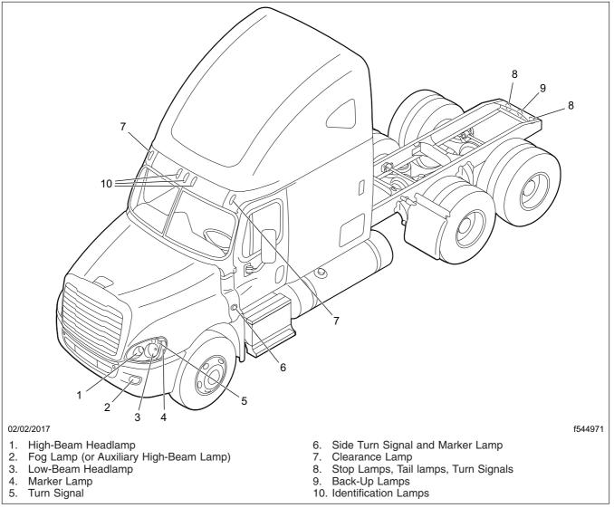
Fig. 21.8, Exterior Lamps
