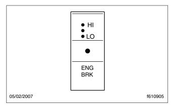
Fig. 5.16, Engine Brake Switch
