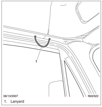
Fig. 5.11, Air Horn Control
