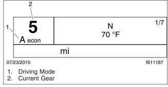
Fig. 15.2, Gear Display Window
