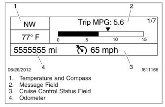
Fig. 4.23, Driver Message Center Without Gear Display, ICU4Me
