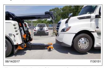
Fig. 24.11, Moving the Stinger and Crossbar Under the Bumper
