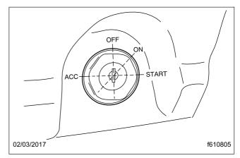
Fig. 25.7, Ignition Switch Positions
