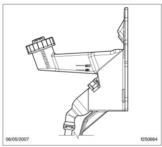
Fig. 14.4, Clutch Fluid Reservoir
