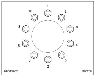
Fig. 21.4, Tightening Pattern, 10-Hole Wheels
