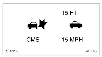
Fig. 6.21, CMS Collision Warning (red)
