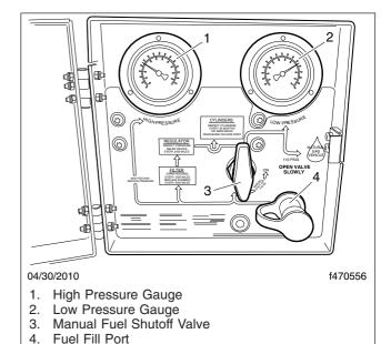
Fig. 21.11, CNG Fuel Panel
