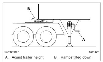
Fig. 18.5, Trailer Connection Point, Low-Lube Fifth
