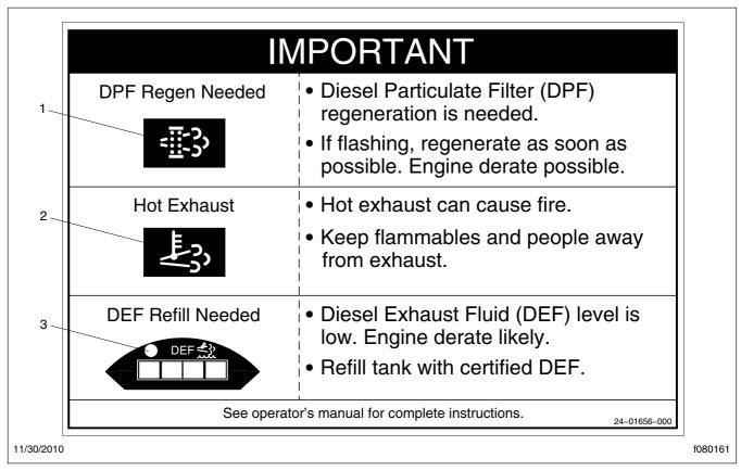
Fig. 12.2, Warning Lamp Decal, Sun Visor
