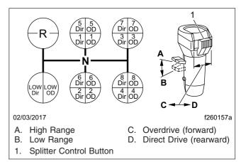
Fig. 14.2, Eaton Fuller 18-Speed Transmission Shift Pattern
